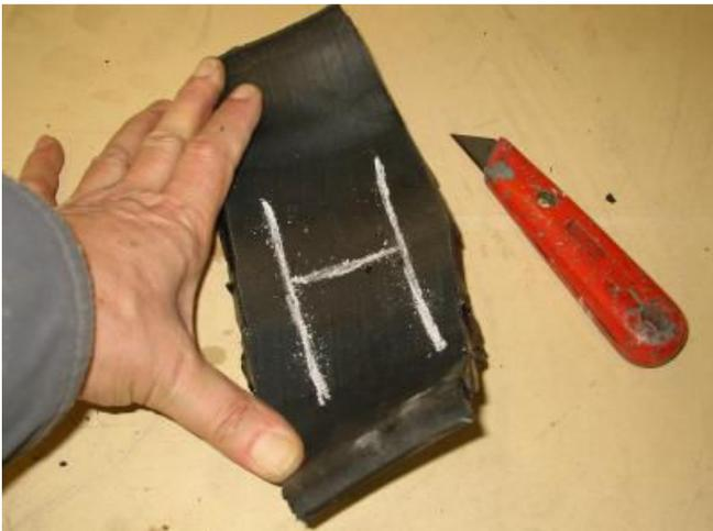
This is the cunning part. Spread open the tyre section and mark an "H", as shown in fig 5. Make the three cuts of the "H" right through the tread, taking care not to sever your thumb at the same time! That completes the "silencer".
