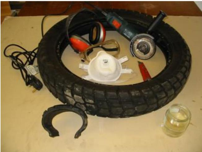
Fig 1 shows what's needed, apart from a piece of chalk, which I forgot, and my trusty old Black & Decker Workmate, which wouldn't fit in the picture. On the left is the safety gear: mask, goggles and ear defenders. The only tools required are a mini-disk angle grinder and a Stanley knife with a new blade. Some might feel happier to include a tape measure even though it isn't necessary, but the jar of water certainly is!
